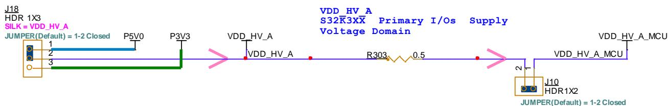
Figure 8. S32K3X4EVB-Q172 | -S172 – VDD\_HV\_A power supply
