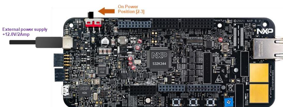
4. When power is applied to the EVB, three orange LED's adjacent to the voltage regulators show the presence of the supply voltages as follows:
