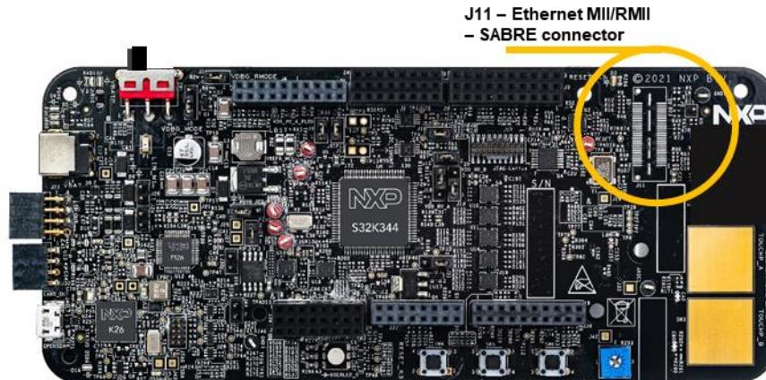
Figure 18. S32K3X4EVB-S172 – Ethernet MII/RMII SABRE connector
