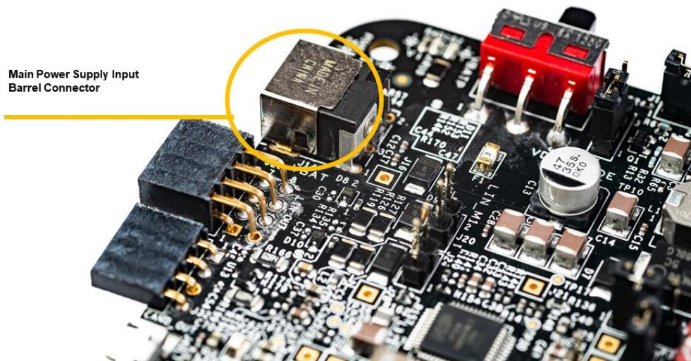
Figure 4. S32K3X4EVB-Q172 | -S172 – Main power supply input
