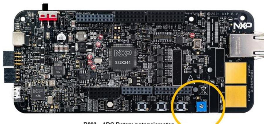
Figure 28. S32K3X4EVB-Q172 – ADC Rotary Potentiometers
