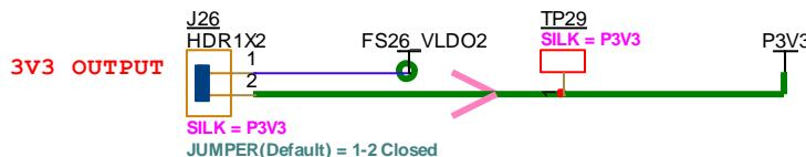
Figure 7. S32K3X4EVB-Q172 | -S172 – General jumper for the P3V3 (+3.3V) reference
