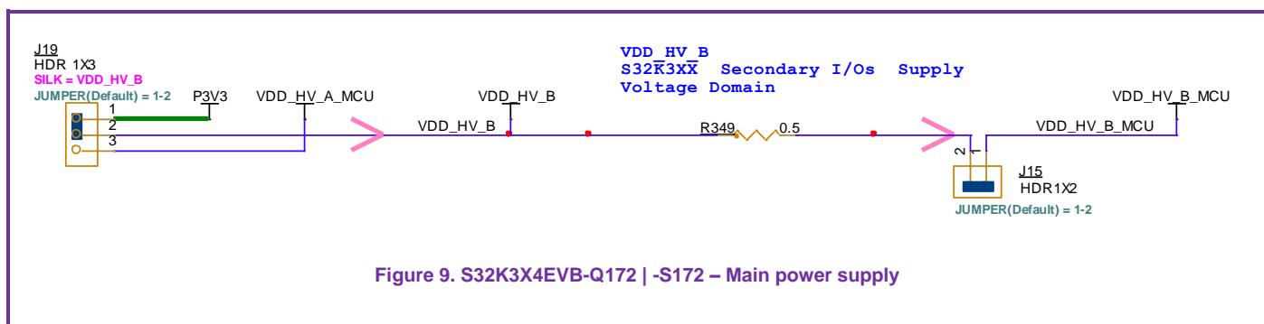
Figure 9. S32K3X4EVB-Q172 | -S172 – Main power supply
