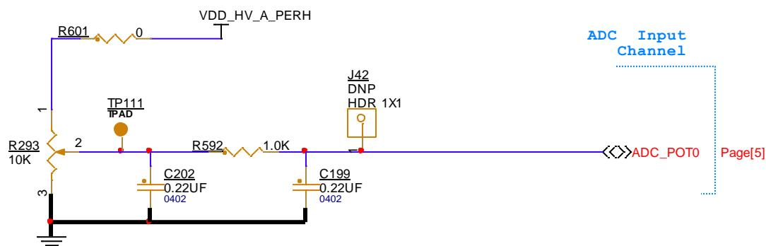
Figure 29. S32K3X4EVB-Q172 – ADC Rotary Potentiometers
