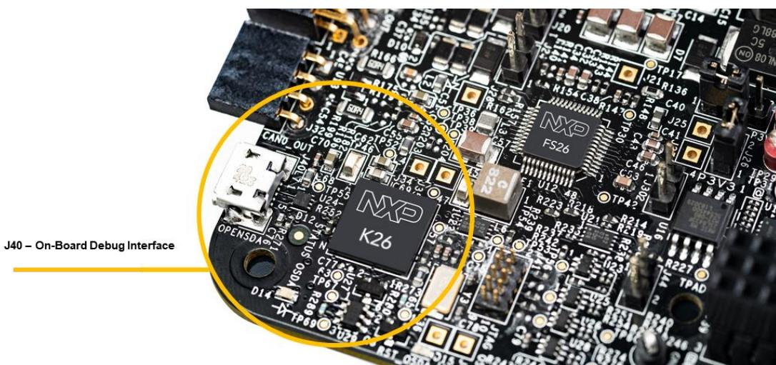
Figure 13. S32K3X4EVB-Q172 | -S172 – On-board S32K3 Debugger
