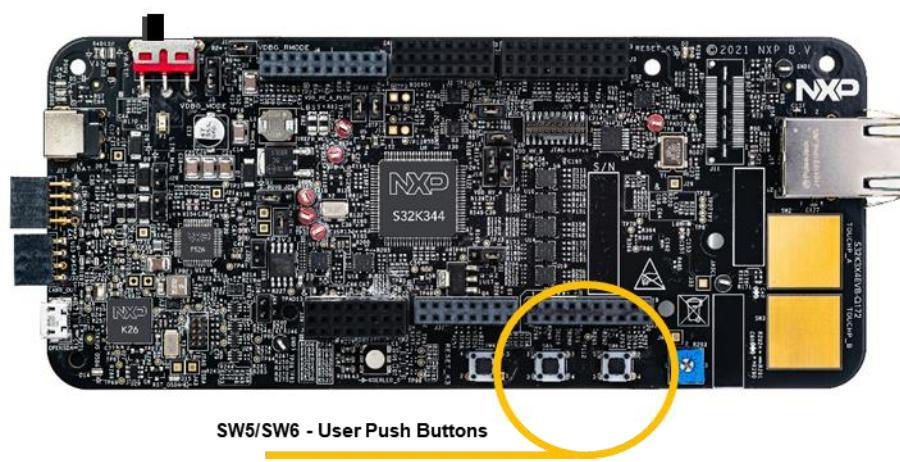
Figure 26. S32K3X4EVB-Q172 – User Pushbuttons
