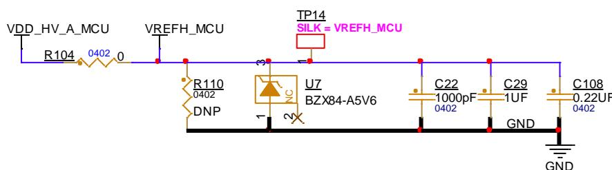
Figure 10. S32K3X4EVB-Q172 | -S172 – VREFH power supply
