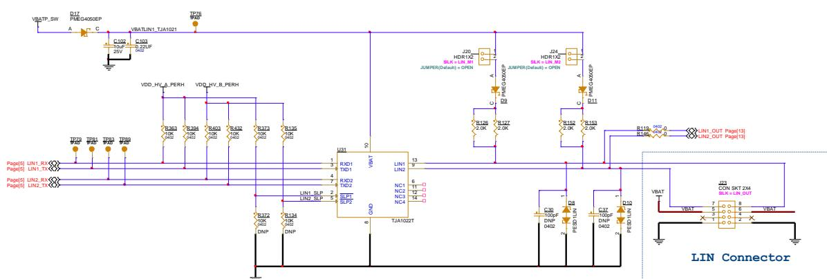
**Figure 15. S32K3X4EVB-Q172 | -S172 – LIN Physical Layer1 TJA1021HG: Quad LIN 2.2A/SAE J2602 transceiver**
