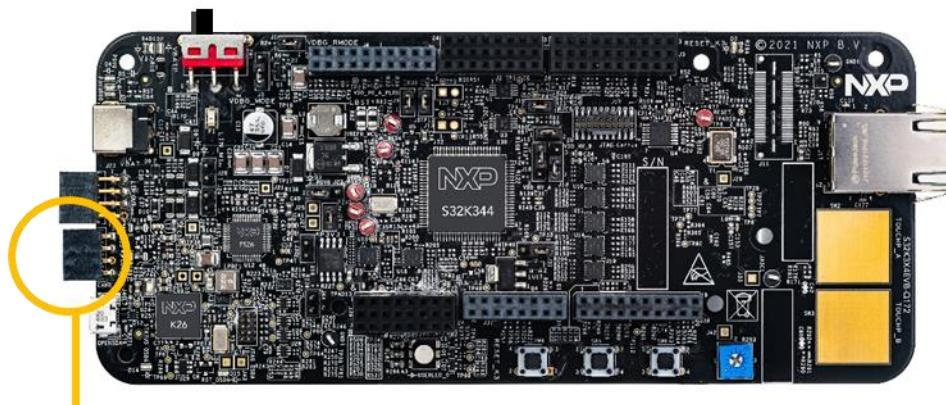
Figure 16. S32K3X4EVB-Q172 | -S172 – CAN Interface
