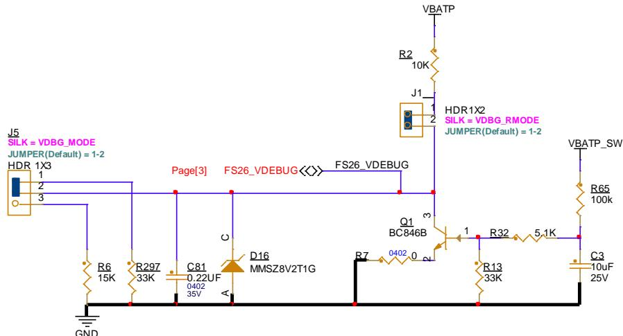
Figure 5. S32K3X4EVB-Q172 | -S172 – FS26/Modes Operation
