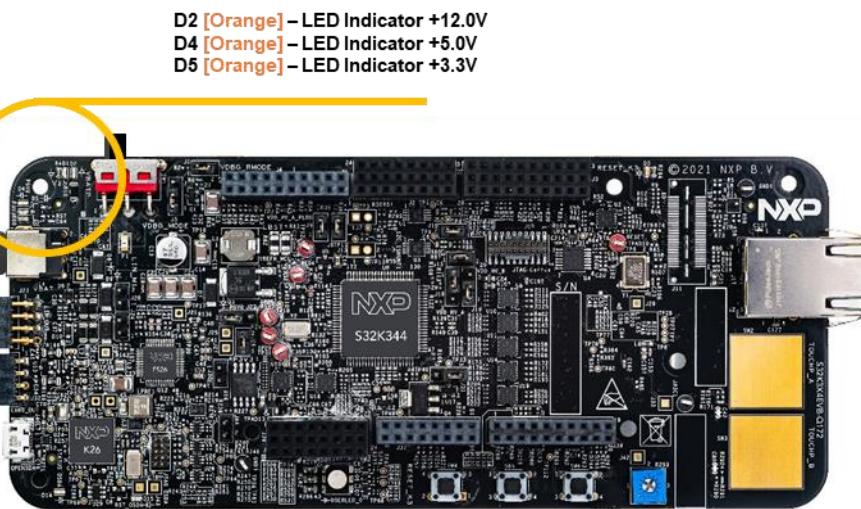
Figure 3. S32K3X4EVB-Q172 | -S172 – Power supply Input and LED power indicators
