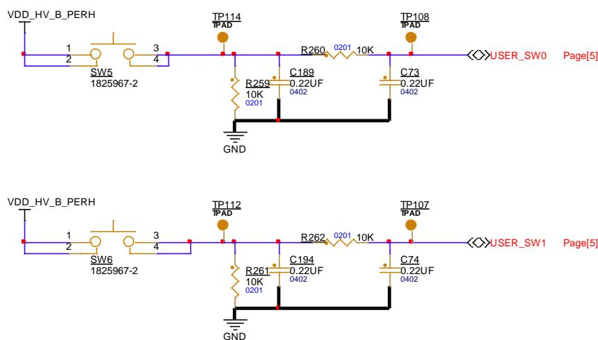
Figure 27. S32K3X4EVB-Q172 – User Pushbuttons
