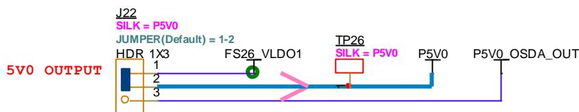
Figure 6. S32K3X4EVB-Q172 | -S172 – General jumper for the P5V0 (+5.0V) reference
