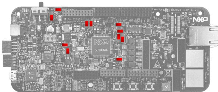
Figure 30. S32K3X4EVB-Q172 | -S172 – Default jumpers' configuration
