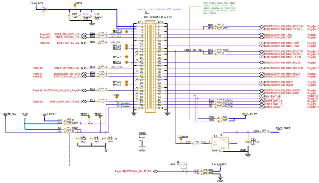
Figure 19. S32K3X4EVB-S172 – Ethernet RMII/MII SABRE Connector
